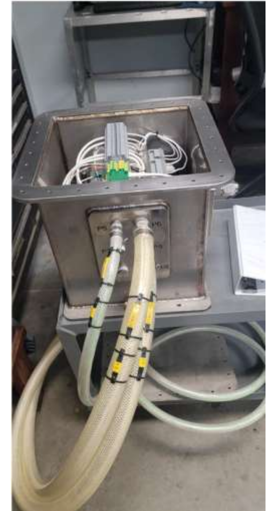
Subsea transformer Tested Pressure balance, oil filled (PBOF) interconnect cables
