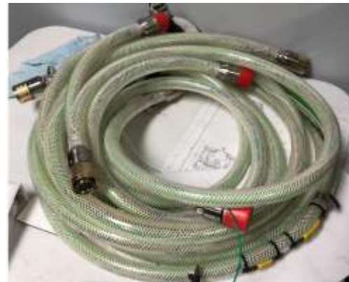
Subsea transformer Tested Pressure balance, oil filled (PBOF) interconnect cables
