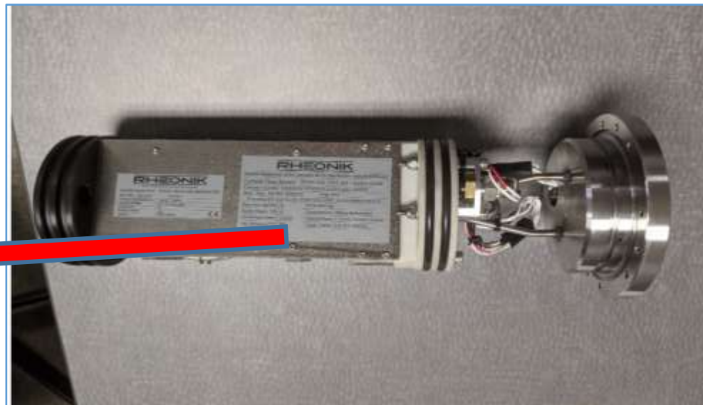
Coriolis Flow meter assembled and tested (w/ Injection pump)
