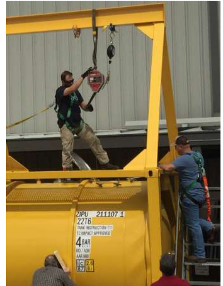
Installing bladder in tank, perfected methodology for installing w/o manned entry
